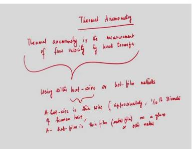
So today, we will discuss about the thermal anemometry. So, this thermal anemometry as I said, this thermal anemometry, this is the measurement, measurement of flow velocity this is by using heat transfers, by heat transfer. Now, so thermal anemometer which are used to measure flow velocity. Now, this is the measurement of flow velocity by heat transfer using either hot film or hot wire methods.
