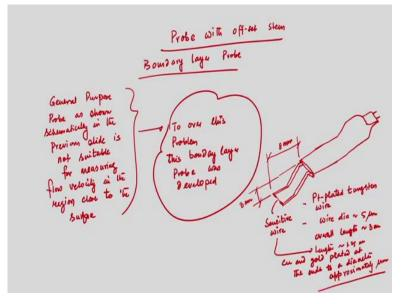
So, probe with offset stem which is also known as boundary layer probe. That means, the general purpose probe, general purpose probe as shown schematically in the previous slide is not suitable for measuring flow velocity in the region, in the region close to the surface. So, to overcome this problem this boundary layer probe was developed.
