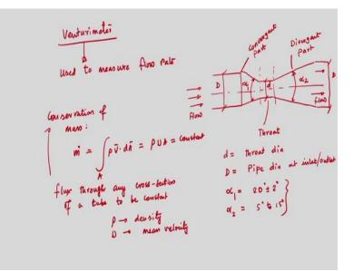
Now, these aspects are also detailed in undergraduate textbooks. In most of the undergraduate textbooks that, you know when you are connecting, you know when you are taking, you know pressure connection to measure the pressure from throat, we need to ensure that the pressure tapings should be connected from, pressure tapping should be taken from those locations where streamlines are perfectly parallel.
