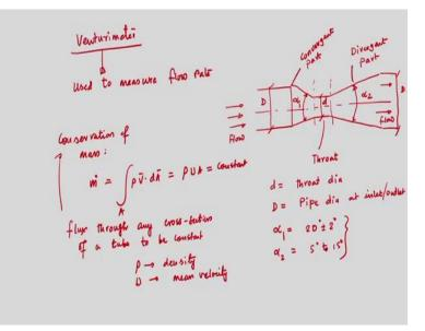
So, see, if we start using venturi meter, in fact, I will discuss only one instrument venturi meter which is used to measure flow rate so, which is used to measure flow rate. So, we know that, this venturi which is used at least to have a drop in pressure of the in the flow field. So, if I try to draw a schematic, which is very simple.
