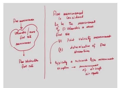
So, I can write the flow measurement is considered to be the measurement of volumetric or mass flow rate, number 1, number 2. It maybe point velocity measurement, or it maybe the determination of flow streamlines. So, when you talk about flow measurement, we are considering either the measurement of volumetric or mass flow rate, that is you know very common as I said, it finds many you know applications, engineering application to be precise.
