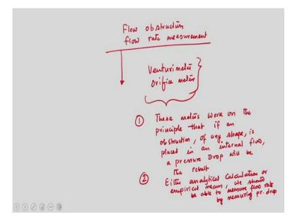
Only thing is 2 important points, that I have written in the beginning that, this flow obstruction fluid measurement techniques because venturi meter, orifice meter and also we will see that another rotavator which you know, works on the principle of drag which is you know, the flow drag.
