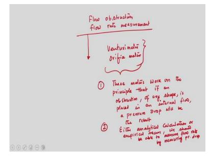
Now so, if I now start our discussion, flow obstruction flow rate measurement. Typically, devices, instruments which are used to measure flow rate following the principle of flow obstruction, in fact I can say those devices or instruments works on the principle of the fact that obstruction of any safe, if it is placed in the flow field, then it will leads to a rise in the pressure, difference, pressure drop.
