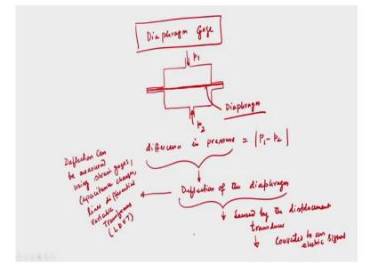
So, I am now drawing the schematic of a diaphragm gauge, diaphragm gauge. If a draw the schematic differential pressure transducer like this. So, we have and so this is say p1 and this is p2 and this is diaphragm, this is diaphragm and so difference in pressure is see p1 minus p2, that is what I said at the beginning that, that is what I said in the beginning that these two gauges work on the principle that there will be a deflection when a pressure difference is applied.
