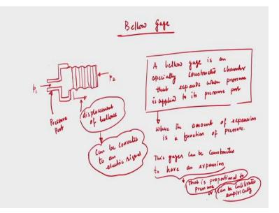
So, bellow gauge again if I draw the schematic then, like this, so this a bellow gauge, this is schematic depiction of a bellow gauge, again we can see that it works on the principle of a displacement or deformation of a structure where you apply pressure difference that is p1 minus p2.
