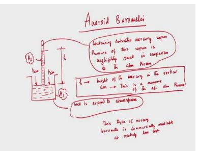
So, today we will discuss about aneroid barometer, I will try to draw the schematic it is a well type manometer. So, this is the schematic depiction, it is having a vertical sealed arm. And now we will try to see the dimension of the sealed arm and what are the other features of this aneroid barometer. Say, this is A1 that is cross section area of the well type manometer well and this vertical height is h. Say, this h is the vertical height of the sealed arm.
