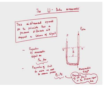
So, the U-tube manometer. So, basically the U-tube manometer is again a type of mechanical pressure measuring device and we have studied in detail about this U-tube manometer in our undergraduate course. And before I go to discuss about U-tube manometer, inclined well type manometer, one thing is important that these instruments operate on the principle that the pressure difference will, is very important support a liquid column of the liquid.
