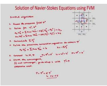
So now, let us write the algorithm whatever we have derived today for the simple algorithm. So first is guess the pressure field P star. Then you solve for U star and V star. So what U star V star so you can write U ae Ue star is equal to summation of A nb Un b star minus delta y Pe minus Pp star with sum source term Bu.
