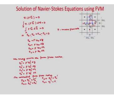
Now, let us write the discrete continuity equation. So, if you see that continuity equation, so it will be divergence of Rho U is equal to 0, so we integrate over the control volume, then you can write divergence of Rho U is equal to 0, dV is equal to 0 and if you convert to the surface integral, then it will be Rho u dot d s is equal to 0.
