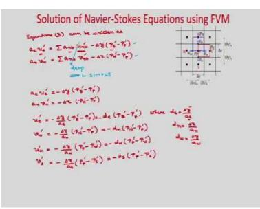
Now equation 3 can be written as. So, now we are introducing the pressure correction and velocity correction. So, it will be Ae U e prime is equal to summation up A nb U nb prime minus delta y Pe prime minus Pp prime. And An Vn prime is equal to summation of anb V nb prime minus delta x Pn prime minus Pp prime. And similar expression may be written for Uw prime and Vs prime.
