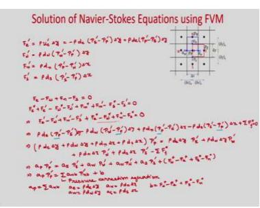
So, now, we will write the corrected mass flow rate Fe prime as Rho e Rho Ue prime delta y. So, now Ue prime you just write in terms of the pressure correction so, it will be minus Rho de Pe prime minus Pp prime into delta y. Or you can write negative sign if you take inside, then it will be Rho into de Pp prime minus Pe prime into delta y.
