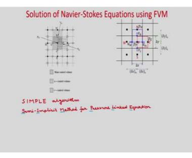
So, you can see that in staggered grid, the pressure is solved in the main control volume. So, you can see this is the main control volume and at cell centre capital P, this Pp is solved. Now, at the face centre of this control volume, small e, now, we have another this red colour cell. So, in that cell we solve for the u velocity for the face centre small e Ue.
