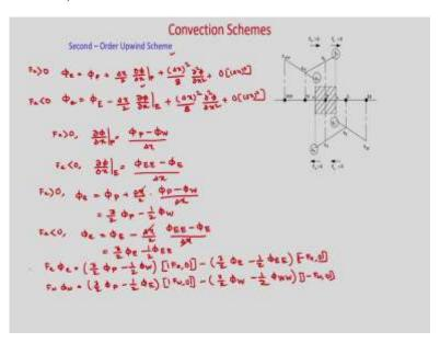
So, now we will use two Second-order upwind points, okay. And it will be Second-order accurate and this is known as Second-order upwind scheme. So, we will use the similar way Phi e we will expand about the point Phi p upwind point, so it will be Phi p plus delta x by 2 del Phi by del x at point p plus delta x squared by factorial 2 and there will be 4, so, it will be 8 del 2 Phi by del x square, okay.
