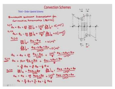
So, this is known as quadratic upstream interpolation for convective Kinematics, okay. So, it is known as Quick and this third-order upwind scheme. So, in this case you can see, to find the value of Phi at the face center e will use two upwind points, if Fe greater than 0 we will use phi p and phi w and one downwind point we will use. So this is your phi e okay it is downwind point.
