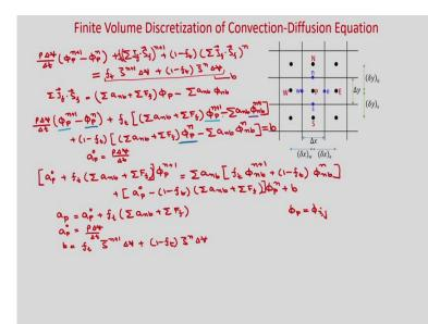
So we have rho delta v by delta t phi p n plus 1 minus phi pn. Then we have summation of Jf dot Sf with a factor Ft and at level n plus 1 and we have 1 minus Ft summation of Jf dot Sf at level n and we have the source term ft S bar n plus 1 delta v plus 1 minus ft S bar n delta. So now, we have already written this term. So, the summation of a Jf, Sf we have written in this form, so, this let us substituted there.
