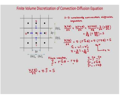
So, 2D unsteady convection diffusion equation. So, in two dimension you can write in conservative form del rho phi by del t plus del rho u phi by del x plus delta rho b five by del y is equal to del of del x gamma del phi by del x plus del of del y gamma del phi by del y plus S. Here, gamma is diffusion coefficient and we have written this convection diffusion equation for any general variable phi and S is the source term and rho is fluid density.
