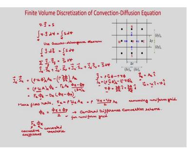
So, first integrate over this control volume so, divergence of j is equal to S where integrating over the main cell P divergence of j dv plus, sorry equal to volumetrical s dv. Now, use Gauss divergence theorem so, you can write integral so, now we are converting the volume integral to surface integral.
