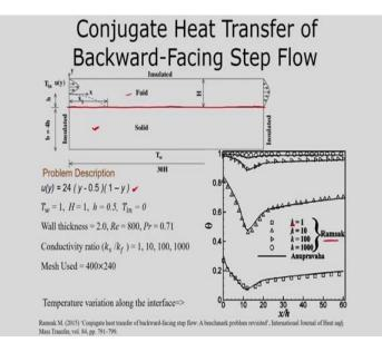
This is a problem of conjugate heat transfer, where in the solid also you solve the heat conduction equation. So, you can see this is the problem, where you have inlet is here and this is the backward facing step and this is the solid.
