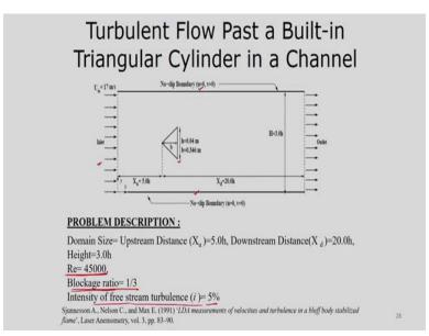
This is a turbulent flow past a built in triangular cylinder in a channel, so this is channel walls, this is your triangular cylinder and you have a inlet velocity and Reynolds number is considered 45000 so that it becomes turbulent and blockage ratio is 1 by 3 and intensity of free stream turbulence is given as 5 percent.
