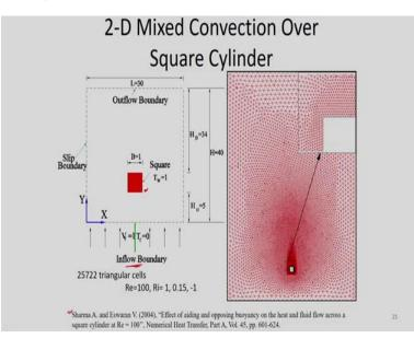
Then this is the problem of Mixed Convection where buoyancy in also included and boussinesq approximation is valid in this case and we have the square cylinder heat square cylinder, heated square cylinder, this is the inflow, so due to buoyancy there will be also there will be buoyancy effect and that we have compared our result with Sharma and Eswaran.
