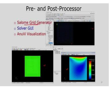
So, these are some snapshots of pre-processors Salome is a grid generator, this is actually open source grid generator and this is the GUI of that, this is the solver GUI and this is the AnuVI GUI, so this is actually post processing solver developed at BARC Bhabha Atomic Research Center at DAE institute.
