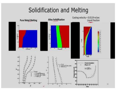
These are some phase change problem, so solidification this is the solidification problem, this is alloy solidification and this is your casting problem, so continuous casting. So, some comparisons are given of these inter-phase when it is moving with time, so that we have compared with the literature.
