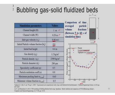
Now, this is the Bubbling gas-solid fluidized bed. So, you have solid particles here and you have some inlet velocity you can see that initial particle volume fraction is given as 0 point 6 and here initial inlet gas velocity as 0 point 46 meter per second and these are the dimensions these are some densities are given and these problem we have solved and compare the time average volume fraction, time average is done between 5 to 60 second of the stimulation time.
