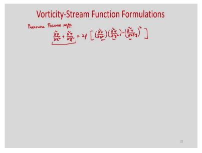
So, this Pressure Poisson equation will look like this but we are not deriving it here, but if you want to calculate, then for this two dimensional situation your pressure person equation will be, del 2 p by del x square plus del 2 p by del y square. So, from the momentum equation you can actually calculate it.
