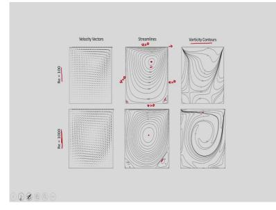
And you print this x, y, u, v, psi, omega to just plot it. So, now you can see the velocity vectors, streamlines and vorticity contours for different Reynolds number. So, Reynolds number 100 and Reynolds number 1000. So, these are the velocity vector u, v we have calculated.
