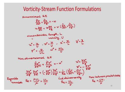
So, our governing equations in dimensional form, dimensional governing equation we have written, del 2 psi by del x square plus del to psi by del y square is equal to minus omega and u del omega by del x plus v del omega by del y is equal to nu del 2 omega by del x square plus del 2 omega by del y square.
