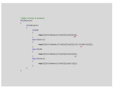
So, next we are actually applying the vorticity boundary condition again. Because psi is applied. So, omega boundary condition will be updated. So, we have updated the boundary conditions.
