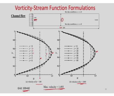
Next, we have solved the channel flow. So, can see, so here L is equal to 6 H we have considered. H is the distance between two plates and u is equal to 1 we have given nondimensional velocity and H we have taken in the Reynolds number. So, we have used grid 100 by 60 and now once you solve and with the, if you solve the vorticity discretize equation and the stream function discretize equation. Along with the boundary condition what we discussed for this channel flow.
