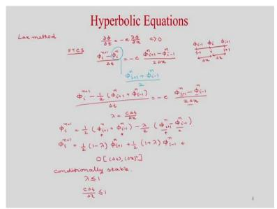
Now, will use Lax method so will start with the forward time and central space. So, with that discretization method and in the time derivative, whatever phi i at time label n will be there that will take the average of phi i n plus 1 and phi i n minus 1. So, if you use FTCS method for the equation del phi by del t is equal to minus c del phi by del x where c greater than 0.
