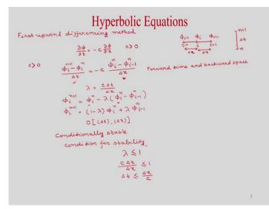
So, now will consider the next method as, first upwind differencing method, first upwind differencing method. So, in this method what will do, depending on the sign of wave speed whether it is c greater than 0 or c less than 0 will choose the scheme. So, same grid will use this is your i, this is your i plus 1 and this is your i minus 1 with uniform step size delta x and this is your delta x, phi i, phi i plus 1 and phi i minus 1.
