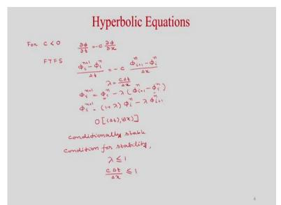
So, now for c less than 0 del phi by del t is equal to c minus c del phi by del x and here now c less than 0 so you use forward in time and forward in space. So, you will get phi i n plus 1 minus phi i n divided by delta t is equal to, minus c phi so forward in space so it will be phi i plus 1 minus phi i divided by delta x with the time label n.
