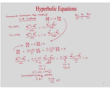
So, these two methods we can combine and we can write in general form which is known as Courant-Isaacson-Ree method, so Courant-Isaacson so these are scientist name Ree method, commonly known as CIR method. So, these two methods will combine and will write in general form using CIR method.
