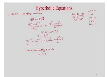
So, this method is known as, Midpoint Leapfrog method so we again will use constant step size. So, phi i, phi i plus 1 and here phi i minus 1 and here we up to now central difference will use in time. So, it will be n minus 1 to n-to-n plus 1 so this is your time step delta t. So, your model equation is del phi by del t is equal to minus c del phi by del x. So, now we will use central difference in time derivative so what will you can write? It will be phi i n plus 1
