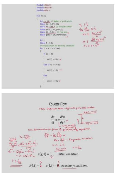
So, you can see in the main function, we have taken total 101 grid points in y direction, so the dx, the distance. The step size we have taken 1 by n minus 1, Reynolds number we have considered 1 and delta t, we have taken 5 into 10 to the power minus 3. So, you can see that what is the condition for stability gamma x is less than equal to half. So, gamma x is you can see, so it is we have different gamma. So, in this case sorry here your gamma will be there.
