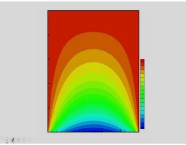
Next, let us consider 2 dimensional unsteady heat conduction equation. So, you can see this is the equation, Del T by Del t is equal to alpha Del 2 T by Del x square plus Del 2 T by Del y square. And let us consider one plate, so this is your bottom wall, this is your top wall, left wall and right all.
