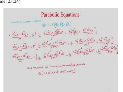
So, we will use Crank Nicolson method in different ways. So you can see, so it will meet Crank Nicolson method, so our governing equation is Del phi by t is equal to gamma Del 2 phi by Del x square plus Del 2 phi by Del y square plus Del 2 phi by Del z square. So, this we can write like phi i, j, k.
