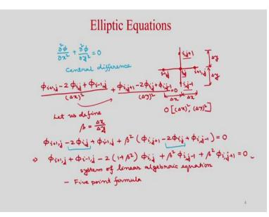
So our governing equation is del 2 phi by del x square plus del 2 phi by del y square is equal to 0. So, this is your governing equation. Now we will discretise this partial derivative using second order accurate scheme, which is known as central difference. So we will use central
