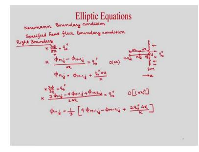
This is also Neumann boundary condition. So, we are considering specified heat flux boundary condition. So, let us consider now right boundary and let us assume that specified heat flux is given at the right boundary. So, if you consider a right boundary, so this is your boundary. Where i is equal to M and let us consider the points at a particular j. So, this is your j.
