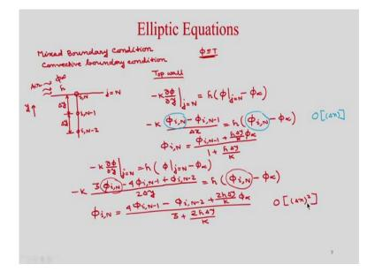
Now let us consider the third type of boundary condition that is your mixed boundary condition and when do we apply this in the heat conduction equation then this is known as convective type boundary condition. So, let us consider a top wall of a solid and that is cooled by a convection. So, if you are considering a top wall, so it is your top wall we are considering.
