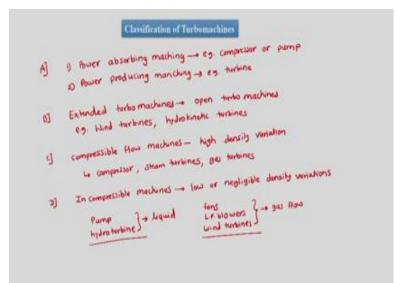
So classification of the turbo machine at the gross would be like we have one a we have first as power absorbing machines. Basically in the power absorbing machines we have fluid which is taking energy from the rotor and we know that example is compressor or pump and second is power producing machines. And in this machines we know that fluid is losing its energy to the rotor and the example is turbine and as what we said they can be any turbine.
