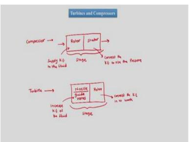
So, let us see what is compressor comprised of. Compressor is comprised of two parts one is called as rotor another is called as stator. So, a flow in compressor will first experience a rotor and then experience the stator then this is called as a stage a combination of rotor and stator is called as a stage. So, if there is a multi-stage compressor then there are multiple pairs of rotors and stators. So, in one stage we have rotor and then we have stator.
