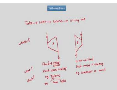
So, the turbo machines whatever we are discussing has a word which is turbo and then this word turbo has latin origin which means turbinis and this turbinis means whirling or spinning top. So, if something is rotating and that something which is rotating for our case are the engine components. But the word here turbo means a rotating top. Now from here we are going to deal with the machines which have rotating components.
