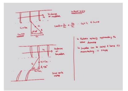
And this is the complete impeller, so we will try how the situation is different, if we are having IGV and without IGV, so this is one impeller, this is other impeller, these are the inducers which we are seeing from the front view and then this is the third impeller, we are plotting inducer of impeller and they are rotating in this direction, we are seeing from the top and then in this case, we do not have any guide vane.
