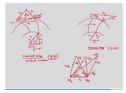
Let us say that now, the blades are not radial, if the blades are not radial, then they can be backward, curved or forward curve, so this is the case where we have backward vanes and in this case, we have velocity triangle and inlet, which is this  $V_1$  velocity and then we have this as radial velocity and so, this is absolute velocity, so we have  $Cr_1$ ,  $V_1$ ,  $C_1$ , so  $C_1$  will make alpha 1 angle, this is complete  $u_1$ .
