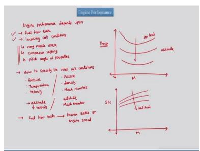
But then, there are certain limitations or certain constraints on increment of the thrust now, we will see engine performance, we have seen till time that propulsive efficiency or cycle efficiency or combustion efficiency overall efficiency, this efficiencies were used by us for the engine performance, here we are trying to see how engine performance is going to alter, which are the parameters governing that and then how it is going to vary with altitude.
