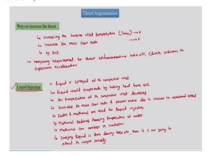
We can increase the thrust of an engine by increasing the turbine inlet temperature, we also call it as T max, if you can increase the T max, then we can increase the thrust, we can also increase the thrust, if we can increase the mass flow rate, so or third option is to increase the thrust by both methods, so this is A, this is B, so by A + B, so we can implement both methods and increase the thrust of an engine.
