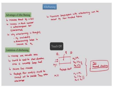
So, advantages of after burning; after burning increases thrust by around 40% however, this increment would further increase with increase in Mach number is advantageous for after burner.
