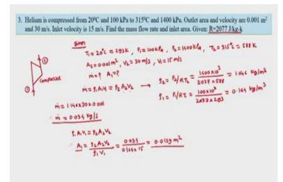
So, we will move next example and next example says that helium is compressed from 20 degree Celsius and 100 kPa to 315 degree Celsius and 1400 kilo Pascal outlet area and velocity are give which are .001 metre square and 30 metre per second respectively inlet velocity is 15 meter per second, find out mass flow rate and inlet area R for helium is given as 2077 joule per kg Kelvin.
