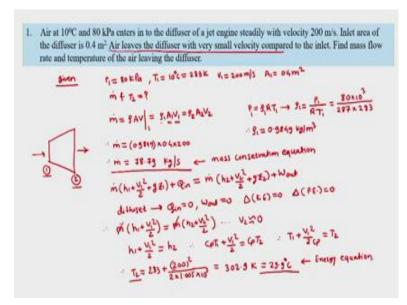
So, the first example says that air at 10 degree Celsius and 80 kilo Pascal enters into the diffuser of a jet engine steadily leave with velocity 200 metre per second inlet area of the diffusion is .4 metre square. Air leaves the diffuser with very small velocity compared to the inlet find out
