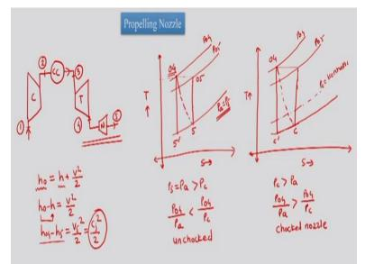
So we know that a typical gas turbine power plant as compressor it as state 1 at the inlet it has state 2 at the inlet then we have combustion chamber after the combustion chamber we have gas turbine which as process 3 to 4 and from the 4 we have nozzle from 4 to 5. So we are talking about process 4 to 5 in the nozzle and objective of the nozzle in general is to act as a duct which would decrease the pressure and increase the kinetic energy.
