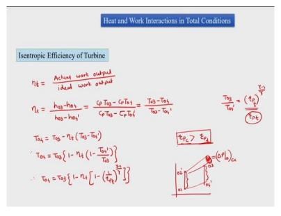
So let us consider the isentropic efficiency of turbine and there we have isentropic efficiency of turbine is equal to actual work output divided by ideal work output now we are trying to represent this in terms of total conditions. So we have
