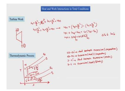
So in case of turbine let us find out the turbine work for that we will again consider the TS diagram in the thermo dynamic process we will consider and then we need to draw 4 lines corresponding to static and stagnation condition. So this is P3 this is P03 this is P04 and this is P4 so for us 3 to 4 dash was the process of isentropic expansion. But now 4 point is brought to 04 and then we get the total condition at 4 point and 3 point is brought to 03 to get the total conditions.
