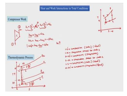
So we know that our Brayton cycle had a compressor which is the first entity and then for the compressor we have process 1 to 2 and the we have 3 to 4 as turbine. So for compressor 1 to 2
