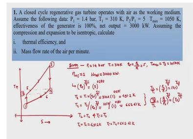
Through examples. For that let us consider the first example it says that there is a closed cycle regenerative gas turbine which operates with air as working medium. So we are given that air is working medium assume the following data P1 is equal to 1.4 bar T1 is equal to 310 Kelvin P2 by P1 is equal to 5 T-max is equal to 1050. Effectiveness of heat exchanger is 100% net power output is 3000 kilowatt.
