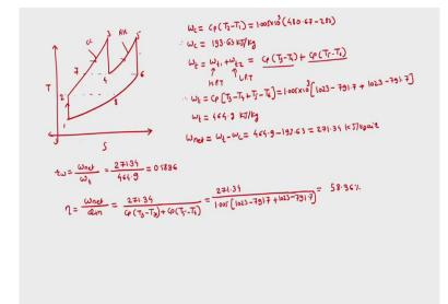
So we move ahead with this given things first we will replot the TS diagram. Such that the numbers will help us 1, 2, 3, 4, 5, 6, 7 and 8 now we can find out compressor work here and then turbine work and then net work for that compressor work it is only one compressor and then there is no mass flow rate is given, so it is specific work output which we can find out
