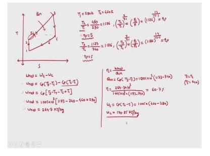
So, we will plot TS diagram for reference we have to keep this point in mind that the regenerator will be ideal if the temperatures are equal we are actually saying it if it has maximum efficiency. So if regenerator works with maximum efficiency with 100% efficiency then the outlet temperature for the heat exchanger in case of air is equal to outlet temperature for the gas in case of turbine. Let us move and then we can say
