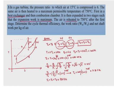
So let us go to the next example, in this example It is told that in gas turbine the pressure ratio to which air at 15 degree Celsius is compressed is 6. The same here is heated to maximum permissible temperature of 750 degree Celsius. First in heat exchanger and then in a combustion chamber so here air is not heated only in the combustion chamber but it is also heated in heat exchanger.
