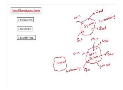
So first is closed system. In case of our closed system suppose this is our system of our interest and then and then this is surrounding in case of closed system we can have certain heat going out of the system certain heat coming into the system. We might have W out of the system. We might have W in to the system but we will not have mass entering into the system. The system which can have interaction with the surrounding in the form of heat and work only is a definition of closed system.
