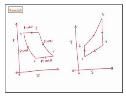
Now the last cycle which is of our interest is Brayton cycle and Brayton cycle is a cycle upon which we have our gas turbine power plant based upon PV diagram for gas turbine power cycle is like this we have 1 to 2 isentropic compression and 2 to 3 constant pressure heat addition, 3 to 4 isentropic expansion and 4 to 1 is constant pressure heat rejection. So this is pressure constant process. This is entropy constant process 1 to 2. This is pressure constant process 2 to 3.
