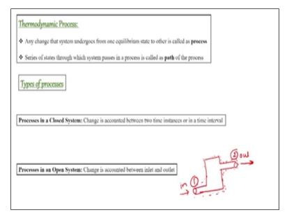
So, any change that system undergoes from one equilibrium state to other equilibrium state system undergoes. So when system undergoes from one state to other state in the previous example, we had said that there is a gas in a cylinder which are certain pressure and temperature at an instance and after certain instance there is certain other pressure and certain other temperature.
