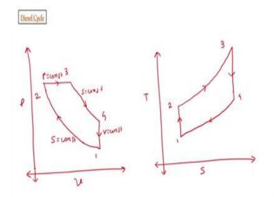
Then next is the Diesel cycle. So for diesel cycle we also know that there is diesel engine and it is also an internal combustion engine. And PV diagram for this diesel engine is like this where we have first 1 to 2 process is same as isentropic compression then at 2 we have constant pressure heat addition from 2 to 3. 3 to 4 is isentropic expansion and 4 to 1 is constant volume heat rejection.
