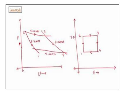
So first cyclic process which you would consider is a Carnot cycle, so let us draw the PV diagram and TS diagram for the Carnot cycle. So, here we will have first PV diagram. Pressure on y axis volume on x axis and as per the PV diagram of this cycle we have process 1 to 2 as the isentropic compression process 2 to 3 isothermal heat addition, process 3 to 4 as isentropic expansion and process 4 to 1 as isothermal heat rejection.
