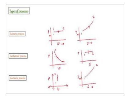
Having said this we have next which is an isobaric process. So isobaric processes as the name suggest is the process where pressure kept constant. So if you try to plot PV diagram then the process 1 to 2 is the isobaric process where pressure is constant. Otherwise if we try to plot TS diagram for the same isobaric process suppose. We are considering heat addition between 1 to 2 this process is like this and if you are considering heat rejection and the processes 2 to 1.
