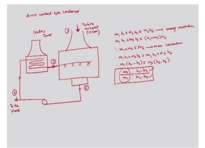
So, first is direct contact type condenser and this condenser looks like this where; so this is state 1, where we are getting turbine exhaust, so this is steam, then this is the cooling water at state 3, it is spread in the air and then this, it is state 2, which is the condensate and then this condensate will be pumped and some will be again circulated in the cooling tower, so here in the cooling tower, this water which is a cooling water will be cooled.
