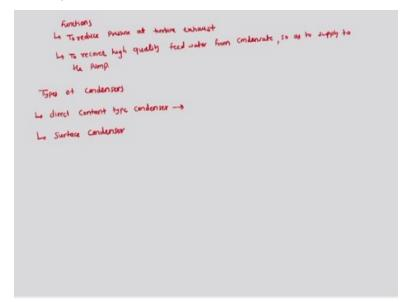
So, condenser; it has following functions; first function is to reduce pressure at turbine exhaust or to keep low pressure at the turbine exhaust, we know that if we keep lower and lower pressure at the turbine exhaust, and more and more expansion can take place for given turbine inlet condition and that will increase the turbine work output, so condenser job is to condense as much low pressure as it can such that we can have higher work output from the turbine.
