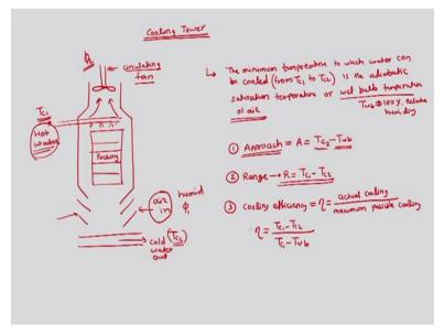
We have seen that cooling tower is a part of condenser and this cooling tower is very much required to cool the cooling water, cooling upon in contact or after having heat transfer from the steam will get heated and that cooling water needs to be re-circulated into the condenser, so we have to remove the heat from the cooling water and that removal of the heat will be taken in the cooling tower, where we will use the atmospheric air to cool the water in the cooling tower.
