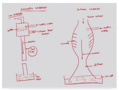
Now, next we can have similar way, one more condenser, again in direct contact type which is called as barometric condenser, this condenser again has direct contact between the steam and the cooling water but here, this mixture is passed through a long tail and that tail will put this mixture into a well, so this is tail and then this is tail pipe and this is hot well and from here, we
