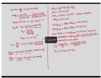
So, friction reduces the velocity so we have  $K_b = 0.85$  and then that is equal to  $\frac{V_3}{V_2}$  and this
