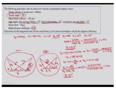
Exit angles are given that is for first row of moving blades, it is given as 18 degree, fixed guide blades it is given as 22 for the exit and second row of moving blades also as exit as 36 degree, steam flow is given as 5 kg per second, blade friction factor is 0.85. Here, we have to remember that we are working with two-stage velocity compounded, so the fixed blades are acting as nozzle.
