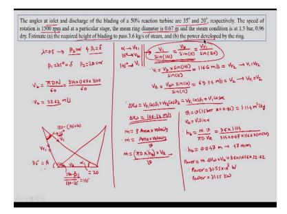
We will move ahead to the next example which states that the angles at inlet and discharge of the blading of a 50% reaction turbine are  $\beta$  are 35° and 20° respectively. The speed of rotation is 1500 *rpm* and at a particular stage, mean ring diameter is given as 0.67 meter. The steam condition is at 1.5 bar, 0.96 dry. Estimate required height of the blading to pass 3.6 kg per second of steam and power developed by the ring.
