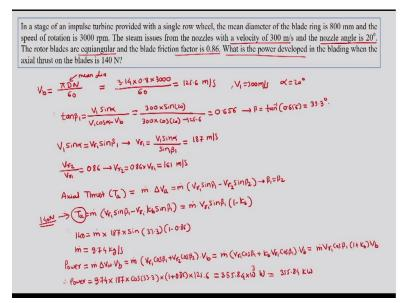
We will see the next example. It reads that a single stage, in a stage of an impulse turbine provided with a single row wheel, the mean diameter of the blade is 800 mm and the speed of rotation is 3000 rpm. The steam issues from the nozzle with a velocity of 300m/s and the nozzle angle is 20 degree. The rotor rotates, the rotor blades are equiangular and the blade friction factor is 0.86. What is the power developed in the blading when the axial thrust on the blade is 140 Newton?
