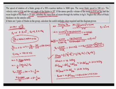
Then, we will go ahead with the next example which states that speed of rotation of blade group of a 50% reaction turbine is 3000 rpm. Mean blade speed is 100 m/sec, the velocity ratio is 0.56 and the exit angle of the blade is  $20^{\circ}$ . If the mean specific volume of the steam is  $0.65 \text{ m}^3/\text{kg}$  and the mean height of the blade is 25 mm, calculate mass flow of the steam through the turbine in kg/sec.
