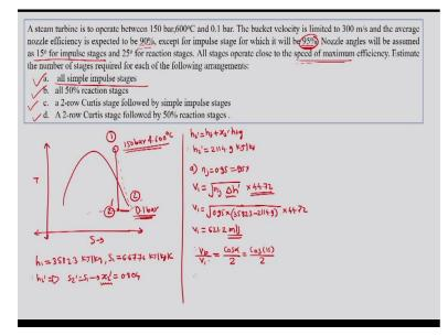
We will move ahead to the next example which states that a steam turbine is to operate between 150 bar,  $600 \,^{\circ}C$  and 0.1 bar. The bucket velocity is limited to  $300 \frac{m}{sec}$ . average nozzle efficiency is expected to be 90%, except for impulse stage for which it will be 95%. Nozzle angles will be assumed as 15° for impulse stage and 25° for reaction stages. All stages operate close to speed of maximum efficiency.
