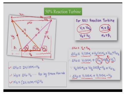
So, now we will move for a particular case of 50% reaction turbine. Now, in case of 50% reaction turbine, we will draw the velocity triangle. So, the velocity triangle is as usual we will have the blade and then there will be velocity which is appearing which is coming into the blade which is relative velocity and then we have  $V_b$  which is blade velocity and then we have  $V_1$ , so as we have drawn the velocity triangles in the impulse turbine.
