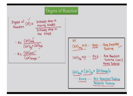
Very first point to be understood here is the degree of reaction. As we have said here that there is enthalpy constant in the moving blades of impulse turbine, but enthalpy decreases so there is an enthalpy drop in case of reaction turbine. So, in case of reaction turbine, we have nozzle and moving blades so there is  $\Delta h$  in the nozzle and then there is  $\Delta h$  in the moving blades, so there is total  $\Delta h$  in a stage.
