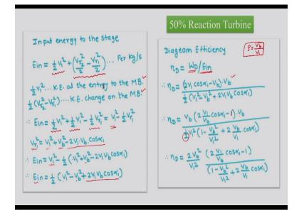
Now, let us find out what is the input energy to a stage. This is very important for us since in case of the impulse turbine, we know that the kinetic energy at the exit of the nozzle is given as an input to the moving blades. So, input kinetic energy was used to divide the work done to get the formula for diagram efficiency. So, diagram efficiency in case of impulse turbine
