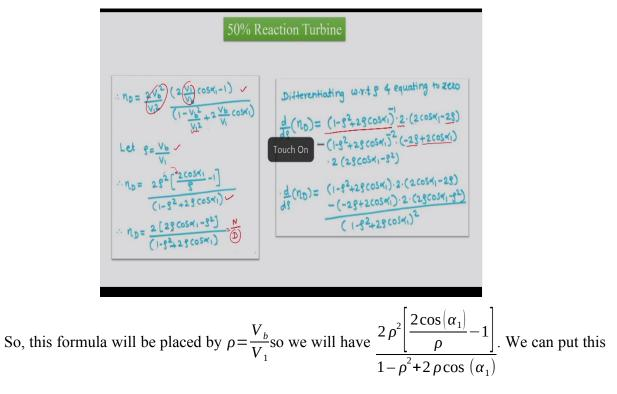
$\rho^2$  into the bracket and then this leads to  $\frac{2[2\rho\cos(\alpha_1)-\rho^2]}{1-\rho^2+2\rho\cos(\alpha_1)}$ . We can differentiate this formula with respect to  $\rho$  and equate it to 0.
