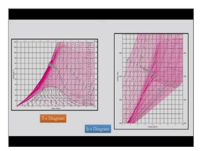
This is a typical T-s and h-s chart from the steam tables. We would need such a steam table to be used for our examples solving or for usage of it when we are dealing with steam turbines or a part of a steam power plant. Then we want here onwards to estimate the properties of practical steam power plant or Rankine cycle.
