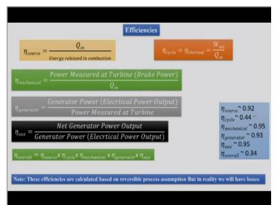
So, then we have efficiencies; then first we have source efficiency( $\eta_{source}$ ) source is something like coal or oil were source efficiency  $\eta_{source} = \frac{Q_{i}}{Energy\,released \in combustion}$  this is source
