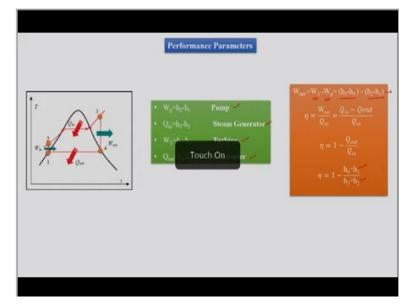
Then once we can know how to estimate all the corners of the cycle like 1,2,3,4 or may be the corners corresponding into saturated conditions. Once we have understanding of this we can point out performance parameters of the steam power plant and those performance parameters initially would include pump work and we have said that pump work is  $h_2-h_1$  across the pump we have enthalpy gain for the water.
