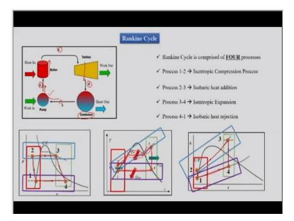
Then how does steam can act as a source where we can use the energy from the steam to generate mechanical energy or mechanical power and hence electricity. We know we have seen in last class that a steam power plant is comprised of four parts. First part is pump where steam would get low pressure to high pressure pumping in the device which is pump. So, steam would get pump from low pressure to high pressure then this process basically is isentropic process.
