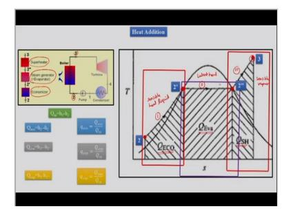
Then we have discussion about heat addition we said that process 2 to 3 is heat addition as what it can be seen here; process 2 to 3 is heat addition process in the boiler. And then, but we know that this is the process 2 to 3 this is process basically. So, the process of heat addition as what we can see it is getting done in the boiler where 2 to 3 is the process of heat addition in the steam power plant.
