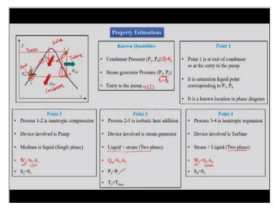
This is our Rankine cycle will typical Rankine cycle there we are saying that we have process 1 to 2 in the pump were we are having work input which is a pump work process 2 to 3 is a heat input in the boiler. So we will say it's a pump here, it's a boiler here, it's a turbine here and it's a condenser here. So, these are the four parts which are dealing with the steam power plant. Now,
