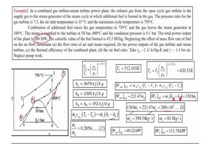
So let us see our next example. And our next example says that, in the combined gas turbine steam turbine power plant, the exhaust gas from open cycle gas turbine is the supply gas to the steam generator of steam cycle at which additional fuel is burnt in the gas. So it is told that exhaust of the gas turbine is first heated by burning extra fuel and then supplied for the supplied as the flue gas in the boiler of the steam power plant.
