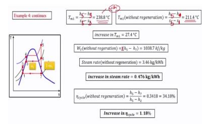
Then this example is continued. We can find out mean temperature of heat addition. Mean temperature of heat addition for the cycle without heat addition and for cycle with heat addition. So mean temperature of heat addition is basically, with
