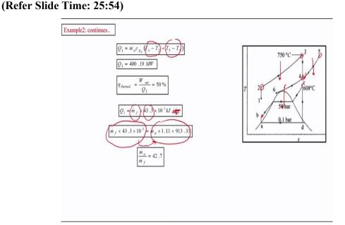
Then we will continue with this example. So we know that now  $Q_1$  is the heat received in the gas turbine and gas turbine is receiving heat twice basically. One is during its combustion chamber and one is before passing it to the boiler, it is also getting heated from 4 to 5. So first heat addition is  $T_3$  to  $T_2$ .  $T_2$ , rise in temperature from  $T_2$  to  $T_3$  and second heat addition is rise in temperature from  $T_4$  to  $T_5$ .
