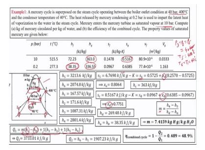
So, this is how we would have solved this example for the regeneration case. Now we will move on to the next example. And next example says that mercury cycle is superposed on the, there is mercury cycle which is superposed on the steam cycle. So mercury cycle is given as a topping cycle and water cycle or steam cycle is given as a bottoming cycle where there is heat exchange between boiler outlet condition at 40 bar and 400 °C and the condenser as 40°C.
