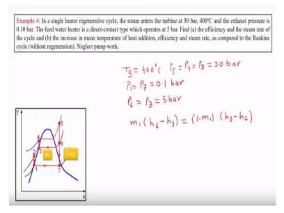
Our first example reads that there is a single reheat regenerative cycle of steam where steam enter the turbine at 30 bar and 400°C. And the exhaust pressure is 0.1 bar. The feed water heater is a direct contact type feed water heater which operates at 5 bar pressure.
