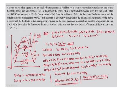
We will move to the next example. This example state that there is a steam turbine power plant which operates on an ideal reheat regenerative Rankine cycle with one open feed water heater, one closed feed water heater and one reheater. The T-s diagram we will draw. Steam enters the turbine at 3 MPa and 400°C and exhausts at 10 kPa.
