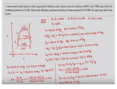
So we are given again in this example that there is open type of feed water heater. So we will again put the same diagram where we have all the time whenever we draw diagram this is an intuition based diagram. This diagram would get corrected based upon the answer. For the example this point, this point 6 we are having at this moment inside the dome. But this might be inside or might be outside the dome.
