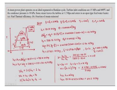
So first example reads as a steam power plant operates on an ideal regenerative Rankine cycle. Turbine inlet conditions are 15 MPa and 600 °C. Condenser pressure is 10 kPa. Some steam leaves the turbine at 1.2 MPa and enters in an open type feed water heater. Find thermal efficiency and fraction of steam extract. So we will start with the given things.
