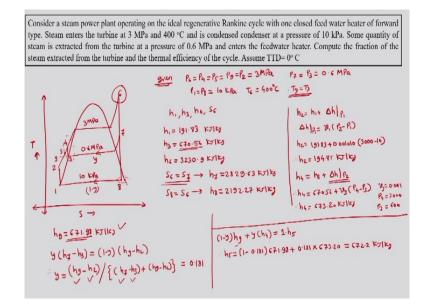
We will go to the next example, which reads that consider a steam power plant operating on the ideal regenerative cycle with one closed feed water heater. The steam enters the turbine at 3 MPa and 400°C and condensed in the condenser at a pressure of 10 kPa. Some quantity of steam is extracted from the turbine at a pressure of 0.6 MPa and enters into the open.
