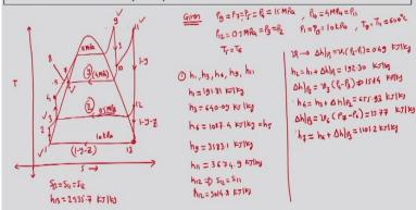
So we will move to the next example. Next example reads that consider a steam power plant that operates on an ideal reheat regenerative Rankine cycle with one open feed water heater, one closed feed water heater and one reheater. Steam enters the turbine at 15 MPa and 600°C and condensed in the condenser at pressure 10 kPa.
