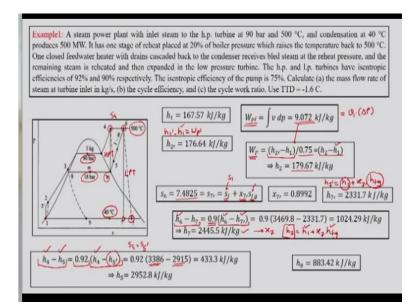
So we know  $P_1$  which is for 40°C saturation condition, so we can go to the steam table, go to the saturation temperature part in the steam table find out 40°C. And then corresponding saturation liquid enthalpy is  $h_1$  and that is 167.57, this is known to us. Then we know that actual pump work is to be evaluated but before that we will evaluate the ideal dash means ideal pump work.
