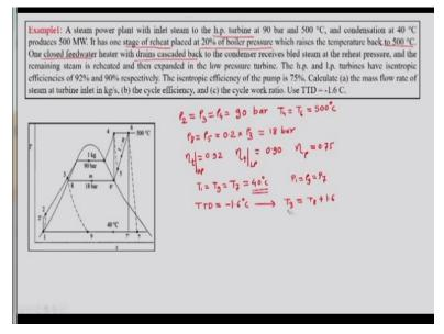
So let us see first example, this example says that steam power plant with inlet steam to the high pressure turbine at 90 bar and  $500^{\circ}C$  and condensation at  $40^{\circ}C$  produces 500 MW of energy. So we are given with 90 bar pressure and  $500^{\circ}C$  are the temperatures of this steam at the high pressure turbine inlet. It has 1 stage of reheat which is taking place at 20% of boiler pressure which rises the temperature back to  $500^{\circ}C$ .
