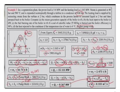
So we can go directly to the steam table at 40 bar and 500 °C and find out  $h_4$  then at the same state we can get the entropy. But this entropy is same as  $S_5$  and  $S_6$  we can use this entropy to find out the condition at 2 bar for the state 5. So what is the enthalpy at 5 we will go to the 2 bar state and then we will find out when this entropy will be equal to  $S_4$  from that we can get the  $h_5$ .
