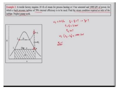
So this is how we would have solve this example and we would have estimated all the necessary parameters. Now let us go to the next example, next example says that there is a textile factory which requires 10 ton of steam per hour for the process heating. So it is a process heating
