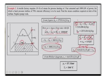
So let us see how we are going to solve this example, so we know that  $h_4$  is a saturation condition and that is at 3 bar. So at 3 bar we can find out saturated steam enthalpy and that is  $h_4$ and then we know that as what we are telling that turbine work is 1000 kilo watt and then that is equal to mass flow rate of steam into change in enthalpy of the turbine. So we know  $h_4$ , we know turbine work and we are also given with the steam which is 10 ton per hour.
