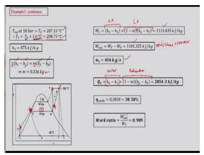
So example 1 is continued, now 18 bar pressure has saturation temperature which is 207.15 °C we had also seen that TTD is given to us. So this is saturation enthalpy saturation temperature + TTD is the temperature at T3. This will be useful to us to find out enthalpy at 3 but this enthalpy is the sub cooled enthalpy corresponding to 90 bar liquid water. This enthalpy would be available again in some steam tables.
