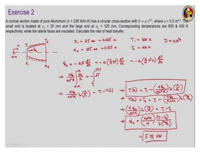
Now let us have the second problem where we have a conical section to deal with, which is made of pure aluminum. Thermal conductivity is given. It has a circular cross section with variable diameter. So the diameter is changing in the direction of heat transfer and accordingly the area corresponding to the direction of heat transfer is also changing.
