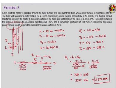
Now let us see one example of applying the cylindrical coordinate system. Again a big problem statement you can pause the video to read it carefully and then again restart the video. A thin electrical heater is wrapped around the outer cylinder outer surface of a long cylindrical tube whose inner surface is maintained at 5 °C. The tube wall has inner and outer radii of 25 and 75 mm respectively.
