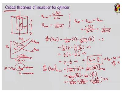
And that is what we are going to identify here in terms of this critical thickness of insulation for a cylinder. As I explained, we have one inner cylinder and this is the outer cylinder. So the inner one is having radius of  $r_1$  outer one is having radius of r. Then our conduction resistance
