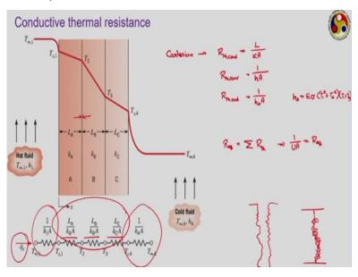
Very similar to the electrical systems, we can consider the given system to be comprising of several such kinds of thermal resistances and accordingly we can form an equivalent thermal resistance circuit and do the analysis. This is called the electrical analogy of heat transfer. Like the situation shown here, from there like yesterday as long as we are sticking to the Cartesian coordinate system, then we can write the thermal resistance for conduction to be
