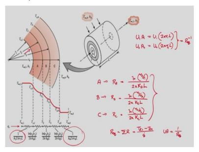
The same thing can easily be extended to the composite cylinder. So when the cylinder is having multiple layers, look at them. There are three layers plus there are two convections on inner and
