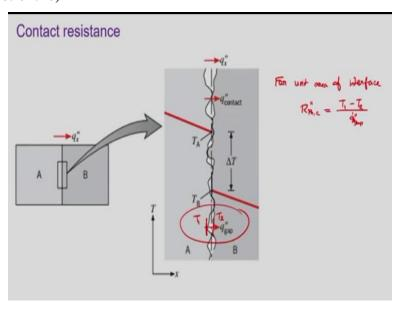
Suppose for unit area of the interface, you are talking about at one point where the temperature is  $T_A$  and another point the temperature is  $T_B$ , then the corresponding thermal resistance at this contact surface will be
