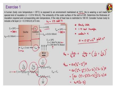
I am not putting the contact resistance in here. I am just talking about thermal resistances. Now, here is my situation. I am talking about a human which is having a body core temperature of 35 °C. He is exposed to an environment maintained at 10 °C. He is wearing a suit made of a special kind of insulation; the corresponding thermal conductivity of insulation for the suit is mentioned.
