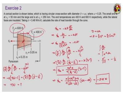
To demonstrate this, I have this problem for you. Here we are talking about a conical section which is having circular cross section in diametereter D = ax. So in the heat transfer direction, this is your x direction,  $x_1$  is this point where the value is given to be 50 mm or 0.05 m, on the other end is 0.25 m. Temperature is given to be 400 and 600 K respectively.
