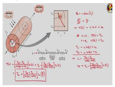
Just like the configuration shown here. Here we are talking about an hollow cylinder or an annular section where the inner radius is  $r_1$ , outer radius is  $r_2$  and we are going to now analyze for this particular one. So we have just seen that
