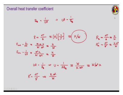
U is the overall heat transfer coefficient and A is the area at which this heat transfer coefficient is defined. As long as we are dealing with planar area like this, the choice of the area does not matter because all surfaces are having the same area.
