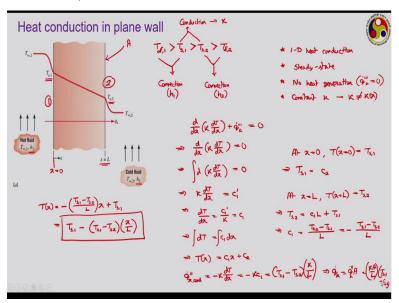
So, we are going to start with heat conduction in plane wall. Plane wall is synonymous to the Cartesian coordinate system and we are talking it as plane wall because the wall, building wall is the most simple example or straight forward example of 1-D heat conduction in Cartesian coordinate. So, look at the situation what is given. We are talking about a wall, let us say this is your x = 0, this is x = L. So, the thickness of the wall is L.
