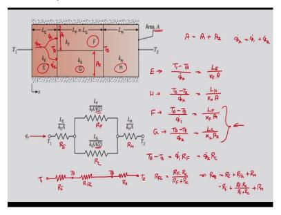
In series connection we have seen that the heat transmission rate through all the resistances will be equal but the effective temperature difference is different, whereas in case of parallel, the temperature difference has to be the same but the heat transmission rate will be different just like shown here. You can think about it is a wall having 3 layers.
