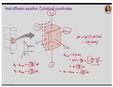
So, first we have the cylindrical coordinate system. This is the problem statement that is given to us. We are having a cylinder just like shown here and we want to estimate or we want to develop the heat diffusion equation inside the cylinder. So, just the same way we have done for rectangular coordinate system from the given domain, we have assumed an infinitesimally small volume.
