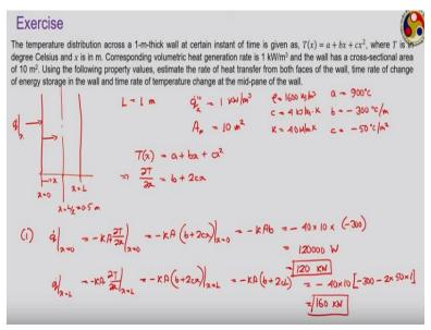
So let us use this idea to solve one exercise problem now. Here the problem is given that the temperature across a 1 m thick wall at a certain instant of time is given. It is given that the temperature distribution is following a quadratic law like this and the corresponding volumetric heat generation rate is given.
