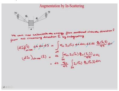
So that will now write. We can now calculate the energy flux scattered into the direction s, from all incoming direction  $s_i$  by integrating. So, in  $dI_{\lambda}$  which is going in direction s, which is your out-scattered should be equal to whatever is coming from all other directions.
