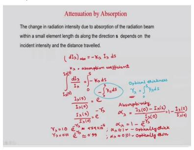
So, let us see that attenuation by absorption. So how the absorption takes place that we have already known that is the Beer's law. So the change in radiation intensity due to absorption of the radiation beam within a small element length ds along the direction s depends on the incident intensity and the distance travelled. So what we can write from the Beer's law? We know that
