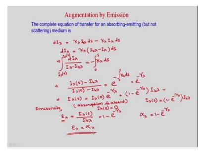
So, now if scattering is absent and only you see absorption and emission, then you can write the complete equation of transfer for an absorbing and emitting medium excluding the scattering as,
