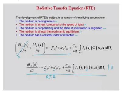
And now, what are the assumptions we have considered during the derivation? Let us summarise. So the medium is homogeneous. The medium is at rest compared to the speed of light, so that I am calling as Quasi-steady. The medium is non-polarising and the state of
