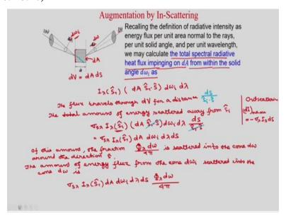
So, we can recall this definition of radiative intensity as energy flux per unit area normal to the rays per unit solid angle and per unit wavelength, we may calculate that total spectral radiative heat flux impinging on dA from within the solid angle  $d\omega_i$ . So we can see this is your ds and this is your dA, so what is the volume of this?
