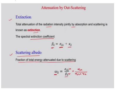
Let us now define what is extinction? Total attenuation of the radiation intensity jointly by adsorption and scattering is known as extinction. So you can see that your attenuation is taking place due to absorption and the out scattering. So obviously, you can see that  $\sigma_{s\lambda}$  is the scattering coefficient and  $\kappa_{\lambda}$  is your absorption coefficient. So, together this is known as  $\beta_{\lambda}$  which is called extinction coefficient.
