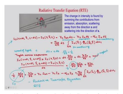
So, now you can see this beam of rays going in the direction of s through this participating medium of distance ds, it is going from s to s+ds, so the distance is ds. And this is the area is dA. The change in intensity is found by summing the contribution from emission, absorption, scattering away from the direction s and scattering into the direction of s.
