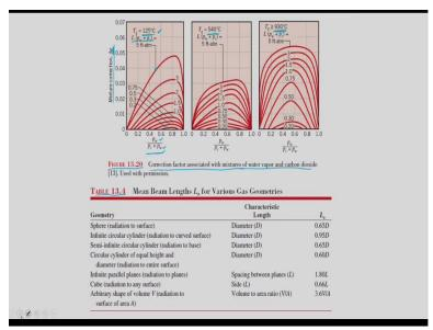
So, that is your figure 13.20 where you will find the mixture correction,  $\Delta\epsilon$ . So, if there is mixture of water vapour and carbon dioxide, then how we will calculate that I will tell in the next slide but before that you need to find the mixture correction factor that is  $\Delta\epsilon$  from this figure and you can see this is correction factor associated with mixtures of water vapour and carbon dioxide.
