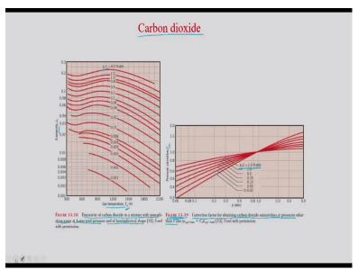
So, this is for carbon dioxide. So, you can see here. So here again it is gas temperature versus emissivity and it is given for 1 atm. You can see emissivity of carbon dioxide in a mixture with non-radiating gases at 1 atm total pressure and of hemispherical volume and also this is given with  $p_cL$ ,  $p_c$  is the partial pressure of the carbon dioxide and L is the mean beam length.
