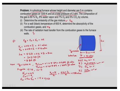
A cylindrical furnace whose height and diameter are 5 m contains combustion gases at 1200 K and at a total pressure of 2 atm. So, you we can see this is one cylindrical furnace, height is 5 m, and your diameter is also 5 m, and it contains combustion gases at 1200 K. So, temperature of the gas  $T_g$  is your 1200 K and total pressure p is 2 atm.
