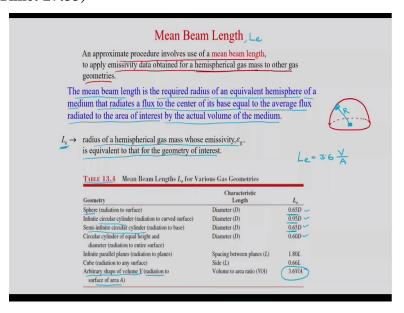
Now, let us talk about mean beam length okay. So an approximate procedure involves use of a mean beam length, to apply emissivity data obtained for a hemispherical gas mass to other gas geometries. So, in general when we study the gas radiation, it is having different geometries. If you consider two plates and in between if you have a participating medium, and you need to find the radiation exchange through this participating medium between these two plates.
