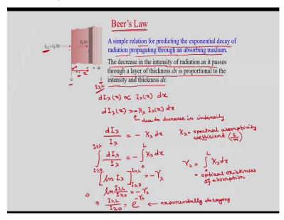
So, first we will discuss Beer's law. Actually, it is a simple relation for predicting the exponential decay of radiation propagating through an absorbing medium. So, we can see this figure. So, some spectral radiation beam of intensity  $I_{\lambda,0}$  actually is incident on the surface where x = 0.
