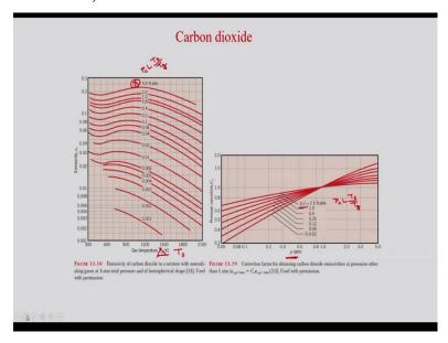
Similarly, in the next figure for carbon dioxide also in place of  $T_g$  you will use  $T_s$ , surface temperature and  $p_c L_e \frac{T_s}{T_g}$  instead of  $p_c L_e$  for both figures 13.18 and 13.19. So, just see x axis is only in atm okay, and the correction factor whatever we have calculated it will remain as it is.
