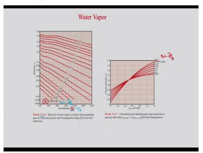
So, if it is 13.16 you can see this is the gas temperature. Instead of gas temperature you use  $T_s$ . So, here you find the surface temperature and that surface temperature you use here along with  $p_w L \frac{T_s}{T_g}$ . So you use  $p_w L \frac{T_s}{T_g}$  instead of  $p_w L$  both in 13.16 and 13.17. So, this is the correction you have to make when you are finding the absorptivity of the medium.
