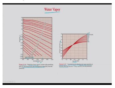
So, this is actually for water vapor. So we can see this figure, figure 13.16. This is actually gas temperature versus emissivity.  $T_g$  is the gas temperature in K versus emissivity. So, if you know the gas temperature then you can find the emissivity and different line you can see, it is for different  $p_wL$  okay. And remember here this unit is given as ft.atm.
