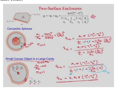
So next, we will consider 2 concentric spheres. So the inner sphere is 1, okay outer sphere is 2 and inner surface temperature is  $T_1$  okay and  $\epsilon_1$  is the emissivity and  $A_1$  is the area, and for outer surface area is  $A_2$ ,  $T_2$  is the surface temperature and the emissivity is  $\epsilon_2$ . So similarly, you find first what is the area ratio  $A_1/A_2$  and what is the area for a sphere, it is  $4\pi r^2$ . So obviously your  $A_1/A_2$  will be
