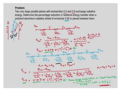
So one problem we are considering that 2 very large parallel planes with emissivities 0.3 and 0.8 exchange radiative energy. So you have 2 parallel plate and they are exchanging the radiation. Determine the percentage reduction in radiative energy transfer when a polished aluminium radiation shield of emissivity 0.04 is placed between them.
