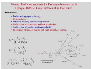
We have considered isothermal and opaque surfaces, then we considered gray surface okay. Then diffusely emitting and reflecting surfaces and surfaces that all experience uniform irradiation as well as surfaces is that all produce uniform radiosity. And also enclosures with gases that do not emit or absorb or scatter. So the gases inside this enclosure does not participate in radiation.
