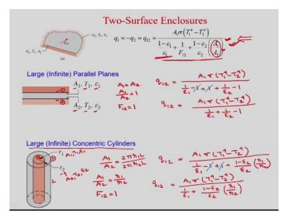
So you can see this are 2 parallel infinite planes okay. So you can neglect the radiation from the 2 ends. So obviously this is the surface 1 okay and this is your surface 2. So this are surface area  $A_1$  maintained at surface temperature  $T_1$  and emissivity is  $\epsilon_1$  and for surface 2, your area is  $A_2$ , temperature is  $T_2$  and emissivity is  $\epsilon_2$ .
