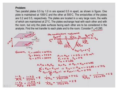
Two parallel plates 0.5X1 m are spaced 0.5 m apart. So you can see these are 2 plates having dimensions of 0.5 mX 1 m and the distance between this 2 plates is 0.5 m. One plate is maintained at 1000 °C and the other at 500 °C. So you can see the upper plate is maintained at 1000 °C and the bottom plate is maintained at 500 °C.
