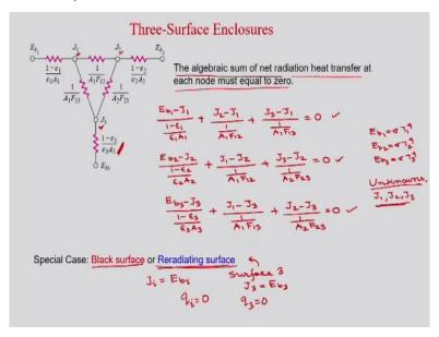
So this is the radiation network, whatever we have drawn right now. So now the algebraic sum of net radiation heat transfer at each node must equal to be 0 okay. So if you consider this node  $J_1$ , so what you can write? You can write
