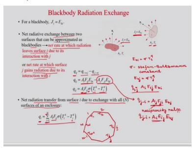
So, let us see first the blackbody radiation exchange. So here you can see in this figure. So it is one surface; isothermal surface maintained at temperature  $T_i$  and area is  $A_i$ . So obviously it will radiate and as it is black surface, there will be no reflection because whatever radiation will come to the surface, all will be absorbed, so there will be no reflection, so the radiosity will be whatever it is emitting only. So, you can see here that
