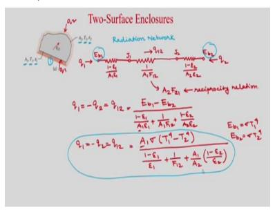
So, first we will consider 2 surface enclosure. So you can see here one surface is this one which is your surface having the area  $A_1$ , constant temperature  $T_1$  and the emissivity is  $\epsilon_1$  and another surface you can see this is your surface  $A_2$ , okay and temperature  $T_2$  and your emissivity is  $\epsilon_2$ . So we can see there will be net radiation exchange between only this 2 surfaces.
