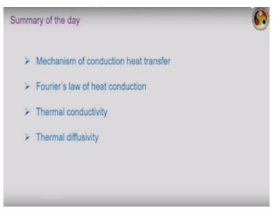
So just to summarize our discussion today, we discussed briefly the mechanism of conduction heat transfer, then the generalised form of Fourier's law heat conduction in three dimensional form in terms of the generalised temperature gradient or acting in that direction normal to an isothermal surface. Then we discussed in detail about the thermal conductivity its contribution coming from the lattice structure and also from the free electrons, particularly in case of solids.
