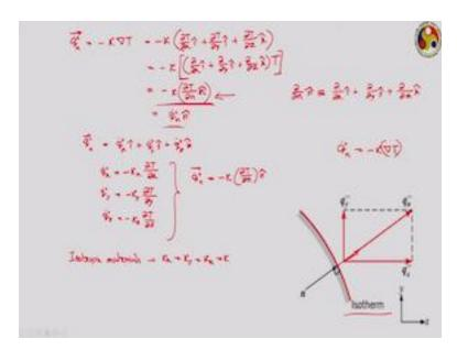
So, we can then write that the generalized form Fourier's law of heat conduction quite often we put a script n to indicate that here talking about heat transfer in this particular normal direction, direction normal to the area is equal to
