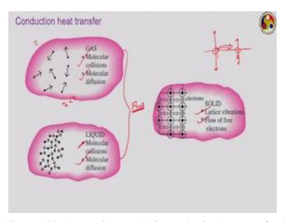
Now, as we have discussed in the previous week, in conduction heat transfer the nature of heat transmission or the primary mode of heat transmission comes from the molecular activity because of the random motion of the molecules in gases, or because of the lattice vibration of the molecules in a solid, we have the energy transmission.
