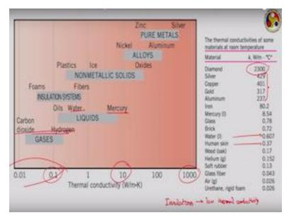
If we just visualize the normal chart of thermal conductivity for different materials; for gases generally the thermal conductivity level is very low just shown here, for liquids we are more on this sides, such as water. Mercury is one of the conducting metals which is remains a liquid state. So its conductivity is significantly higher. Look at the level, for mercury it is  $10~\rm W/m.K$ , whereas for gases of hydrogen etc it is just 0.1.
