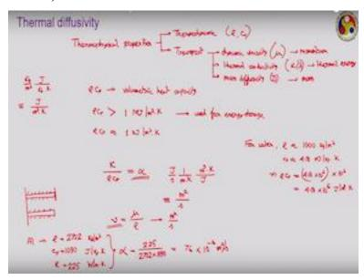
There is another property that is also very important that is called the Thermal diffusivity. Now the thermo physical properties for any matter are generally classified into two categories. So thermo physical properties can be classified as one group, which we call the thermodynamic properties and other is the transport properties. Thermodynamic properties referred to properties like density, specific heat, which are used extensively in thermodynamic analysis.
