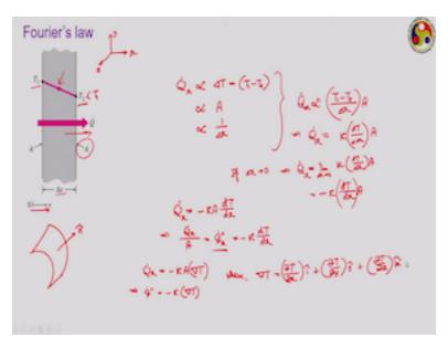
Next is the Fourier's law of heat conduction, which I have already introduced, but I am now trying to go into a bit more detail on that. Here, I am showing you one block. Just assume it's a block of some thickness  $\Delta x$  and its dimensions in the other two directions are extremely large. Let us apply a coordinate system somewhat like this. Say, this is our x direction, this is our y direction and this is the z direction.
