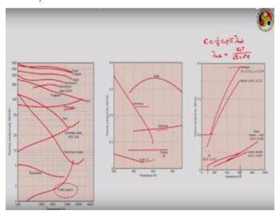
Now this is a chart which shows the temperature dependence of thermal conductivity for solids. As the temperature increases, the electronic movement part that does not get affected that much. But lattice structure, the  $K_{lattice}$  part generally keeps on reducing. Accordingly you can see there is a little bit of reduction for most of the materials thermal conductivity. But exception can be platinum at high temperature or certain kinds of quartz.
