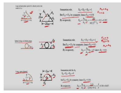
So this is the configuration, long inclined plates point B is directly above the centre of  $A_1$  okay. So this surface is  $A_1$  and if its centre is this one, B is just above this centre okay. And the dimensions are given. So this distance from the centre to B is 100 mm and this  $A_1$  is 200 mm
