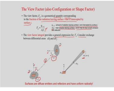
It is also known as configuration factor or shape factor. So you can see the slide the view factor  $F_{ij}$  is a geometrical quantity corresponding to the fraction of radiation leaving surface i that is intercepted by surface j. So if we consider two surfaces, from one surface to another surface, your radiation will go. So whatever radiation actually living surface i and what is the fraction of it actually reaches to the surface j that is known as the view factor.
