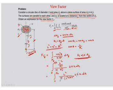
So I am first reading the problem. Consider a circular disc of diameter D and area  $A_j$  above a plane surface of area  $A_i$  ( $\ll A_j$ ). So  $A_i$  is the surface which is very small surface compared to the surface  $A_j$ . The surfaces are parallel to each other, and  $A_i$  is located at a distance L from the centre of  $A_j$ . So obviously these two disc are kept parallel and the distance between these two centres is L. Obtain an expression for the view factor  $F_{ij}$ .
