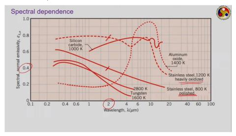
Spectral dependence is shown here for certain common material. You can see there is no specific trend in materials like stainless steel, tungsten, etc.; their spectral normal emissivity that is. Now
