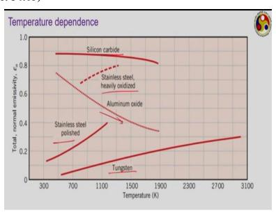
This is the temperature dependence for certain common materials again. You can see for materials like tungsten or polished stainless steel, even oxidized stainless steel also, it increases with increase in temperature the total normal emissivity. For silicon carbide it is more or less flat
