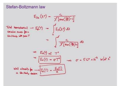
Now, we know the spectral hemispherical emissive power for a black surface. Then let us try to calculate the value of total hemispherical emissive power. So we have just seen that the spectral hemispherical emissive power  $E_{\lambda,b}$  corresponding to  $\lambda$  T,
