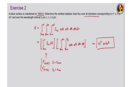
And another problem let us very quickly solve it to wrap up the chapter. We have a black surface maintained at this temperature. We have to determine the emitted radiation heat flux over all directions corresponding to  $\theta$  equal to 0 to 60 and  $\lambda$  equal to 2 to 4 micron okay. Here all directions actually refer to all directions of  $\varphi$ . But  $\theta$  variation is there. So you have to calculate the radiation heat flux.
