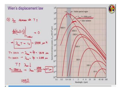
Now, if we plot this  $E_{\lambda,b}$  with  $\lambda$  for a given temperature, then this is what we are going to get. Here we have the wavelength  $\lambda$  and this is the spectral hemispherical emissive power for a black surface  $E_{\lambda,b}$ . Often for black surface or black body, so we do not mention the hemispherical term because it is a diffuser emitter. So by default it is always giving you hemispherical idea.
