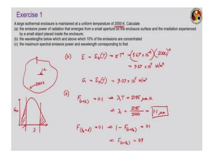
And that is what we are getting finally as the simple form in terms of Stefan Boltzmann law. So, I shall be rounding off quickly by solving 2 numerical problems. First one is corresponding to a large isothermal enclosure maintained at a uniform temperature of 2000K, so we have a large enclosure maintained at a uniform temperature of 2000K. Several things we have to calculate, first the emissive power of radiation that emerges from a small aperture.
