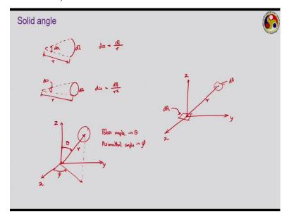
If suppose we are talking about a 2D space and this is one arc and this is one point, then if we join the end of the arc by these lines to this and then if the length of this arc is dl and this angle is equal to  $d\alpha$  and the radius of this arc is equal to r, then we know that we can relate this  $d\alpha$  with this dl as
