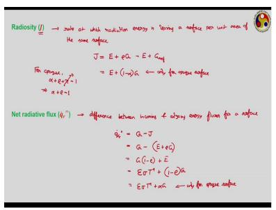
Next, we define a parameter called radiosity. Radiosity refers to total amount of energy leaving the surface. Here, look at this the emissive power is defined as the rate at which radiation energy is emitted by a surface. Whereas for radiosity, we define this one as rate at
