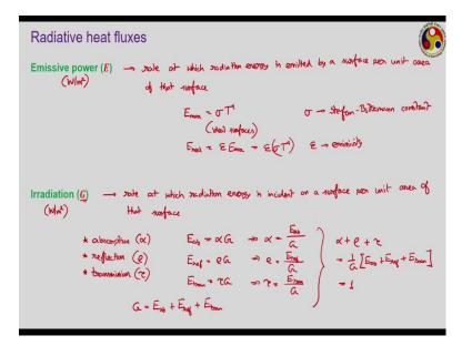
Now, you have to define the radiative heat fluxes. There are 4 different radiative heat fluxes that we need to know. The first one is emissive power that E that I am talking about. Emissive power refers to the total amount of energy leaving the surface per unit surface area. So, emissive power can be defined as the rate at which radiation energy is emitted by a surface per unit area of that surface.
