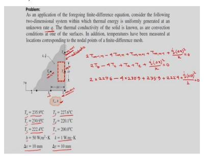
So you see this problem. As an application of the foregoing finite difference equation, consider the following two dimensional system within which thermal energy is uniformly generated at an unknown rate  $\dot{q}$  okay. The thermal conductivity of the solid is known as are convection condition at one of the surface. In addition, temperatures have been measured at location corresponding to the nodal points of finite difference mesh.
