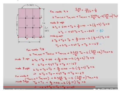
So boundary points if you remember, we have already done for a flat surface with heat convection. So we can write for node 3 and 6. So for node 3 and 6 we can write
