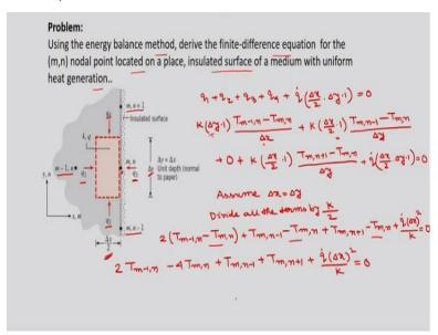
So let us solve the next problem. Let me read first. Using the energy balance method derive the finite difference equation for the (m, n) nodal point located on a place, insulated surface of a medium with uniform heat generation. So in this case we are considering uniform heat generation and the boundary surface is insulated that means it is adiabatic boundary condition and there will be no heat transfer across this boundary okay.
