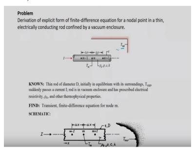
So at last now we will solve this unsteady heat conduction problem. So you can see the problem is derivation of explicit form of finite difference equation for a nodal point in a thin electrically conducting rod confined by a vacuum enclosure. So there is a vacuum enclosure you can see
