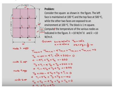
You see here, consider the square as shown in the figure. The left face is maintained at 100 °C and the top face at 500 °C while the other two faces are exposed to an environment at 100 °C.
