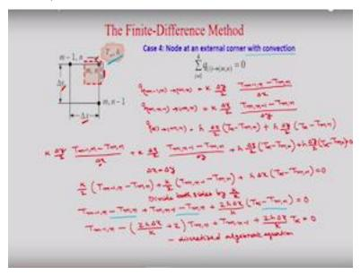
So that is your node at an external corner with convection. So you can see here, it is an external corner node,  $T_{m,n}$  and this side and this side are open to atmosphere and heat convection is taking place there, with ambient condition  $T_{\infty}$  and h okay. So in this case let's derive the heat transfer rate from (m-1, n) to (m,n). So area in this case it will be half okay. So it will be  $\frac{\Delta y}{2}$ , and the distance will be  $\Delta x$  okay. So it will be
