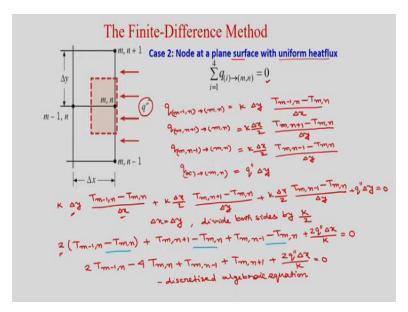
So now another type of boundary condition we will consider for a node at a plane surface with uniform heat flux okay. So you have a plane surface where uniform heat flux is there. So you can see uniform heat flux q'' we are considering on this surface okay, so for this particular nodal point (m,n) we will write
