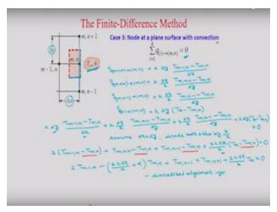
Now you consider node at a plane surface with convection. So this is your plane surface and this is open to convection okay.  $T_{\infty}$  and h okay. It is not a corner point. It is a plain surface and the heat convection is taking place. So heat transfer coefficient is h and temperature is  $T_{\infty}$  and it is obviously boundary points at  $T_{m,n}$ . So at this point now how we will find that temperature. So we will use same energy balance okay.
