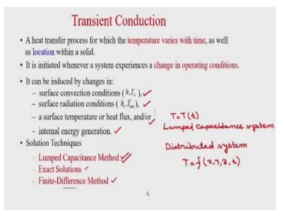
So a heat transfer process for which the temperature varies with time as well as location within a solid is known as Transient Conduction. So there may be two possibilities. One is temperature may vary only with time okay. So your T may vary only with time okay, but there will be no spatial variation of temperature okay, so that is known as Lumped Capacitance System; where everywhere inside the solid temperature will be same.
