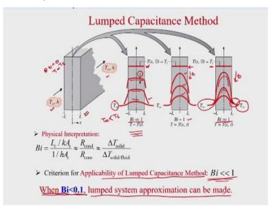
So we will go to the next slide. So now let us consider one plane wall and symmetrically your convection is taking place from both the sides and we will see for different Biot number what will be the temperature distribution inside the solid. So we have considered one plane wall both sides we have same condition, convection condition h and  $T_{\infty}$ . So now let us consider where Biot number << 1 where internal resistance you can neglect.
