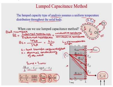
So we already told that the lumped capacity type of analysis assumes a uniform temperature distribution throughout the solid body okay. So when can we use lumped capacitance method? So when this lumped system analysis is valid? It is actually determined by one non dimensional number which is known as Biot number. So this Biot number actually determines whether you can use the lumped capacitance system method or not for the solution of the temperature in a solid.
