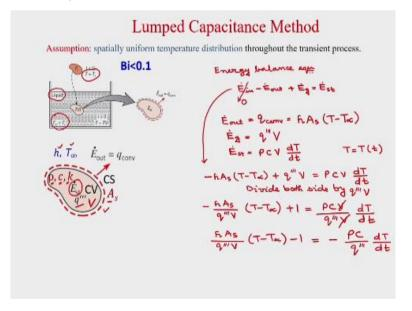
Now we will consider lumped capacitance method where temperature varies with time only. That means we will consider Biot number < 0.1 and in a generalized way we will derive the temperature distribution of the body. So actually how temperature varies with time that we will find in this case. So let us consider a solid body okay, or solid metal body solid metal forging which was initially temperature at  $T_i$ , initially it was very hot and its temperature is
