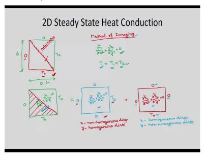
So, let us consider one right angle triangle like this okay. Third direction is infinite, so we are considering a two-dimensional case. So it is a bar of triangular cross-section okay right angular cross-section. Now, the hypotenuse is maintained at adiabatic condition. Adiabatic means there will be no heat transfer across the surface, okay. And let us say base is maintained at  $T_0$  okay, and the height is maintained at 0 okay. So, method of imaging we will use to solve this problem.
