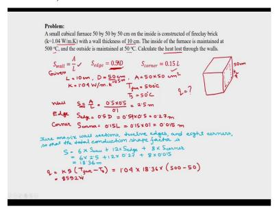
So, I am reading this problem. A small cubical furnace  $50 \times 50 \times 50$  cm on the inside is constructed of fireclay brick of thermal conductivity 1.04 W/mK with a wall thickness of 10 cm. The inside of the furnace is maintained at 500 °C and the outside is maintained at 50 °C. Calculate the heat lost through the walls.
