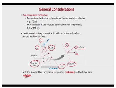
So, let's consider this figure where T is function of (x, y) and top and bottom walls are adiabatic. Adiabatic wall means no heat loss okay. So, through these walls, there will be no heat loss okay. So, now left wall is maintained at temperature  $T_1$  okay and this slant right
