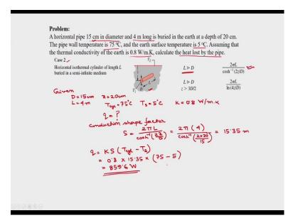
So, I am reading the problem first. A horizontal pipe 15 cm in diameter and 4 m long is buried in the earth at a depth of 20 cm. The pipe wall temperature is 75 °C and the earth surface temperature is 5 °C. Assuming that the thermal conductivity of earth is 0.8 W/mK, calculate the heat lost by the pipe. So, in this case  $T_1$ ,  $T_2$  are given, k is given. And for this particular case we have to find the conduction shape factor and the heat transfer rate q.
