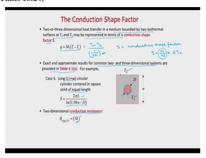
So, now we will introduce using this approach the conduction shape factor. So, what is conduction shape factor? Generally two and three-dimensional heat transfer, in a medium bounded by two isothermal surfaces  $T_1$  and  $T_2$ , maybe represented in terms of conduction shape factor S.
