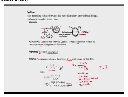
Now, we will solve some problems to understand this graphical method as well as we will use the shape factor here. So, one case you just see, one heat generating radioactive waste is there okay which is actually generating heat okay with  $\dot{E}_g$  of 500 W. So, we have to find the container surface temperature  $T_1$  where z from the surface it is kept at distance 10 m. This surface is maintained at temperature  $T_2 = 20$  °C.
