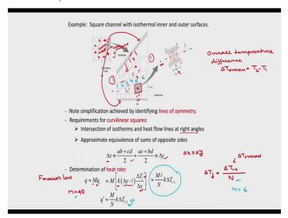
So, you can see this is a square channel with isothermal inner and outer surface. So, you can see this is your inner surface and this is outer surface okay. So, we are considering a two-dimensional square channel and inner surface is maintained at temperature  $T_1$ .
