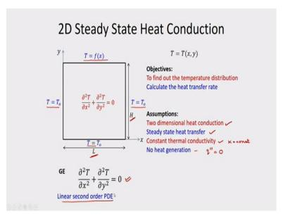
So let us consider two dimensional plate okay. So here you can see it is a two dimensional plate of length L and height H okay. So it is a rectangular plate and of length L and height H. And we need to find the temperature distribution inside this plate. So what are the objectives? Objectives are to find the temperature distribution and once we find the temperature distribution we need to find the heat transfer rate.
