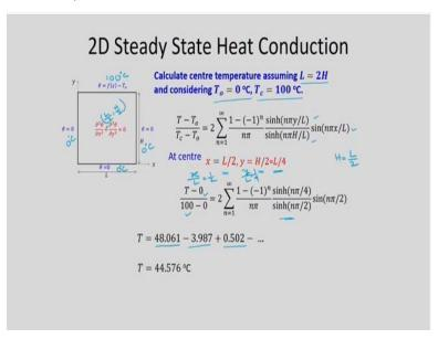
Then we will find that within three values it will converge. So if you see this is the problem where calculate centre temperature assuming L = 2H okay and considering  $T_0$  as 0 °C and  $T_c$  is 100 °C okay. So here it is 100 °C okay on the top. And this is 0 °C. This is also 0 °C and this is also 0 °C okay. So with this condition and L = 2H.
