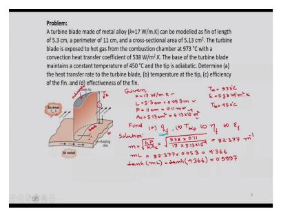
So, first I will read the question. A turbine blade made of metal alloy where k is 17 W/mK can be modeled as fin of length of 5.3 cm, a perimeter of 11 cm and a cross-sectional area of 5.13 cm<sup>2</sup>. The turbine blade is exposed to hot gas from the combustion chamber at 973 °C with a convection heat transfer coefficient of 538 W/m<sup>2</sup>K.
