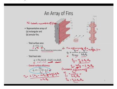
And you can see this is array of fins, so this is your array of rectangular fins and this figure is your array of annular fins. So, there are many fins are there. So, these fins are connected with the base surface and here let us say that if you have N number of fins, then what will be their total surface area?
