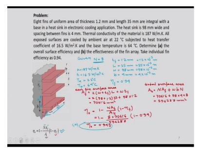
So, in the last problem let me first read out. Eight fins of uniform area of thickness 1.2 mm and length 35 mm are integral with a base in a heat sink in electronic cooling applications. So, you can see that it is the case of an array of fins because here you have total eight fins okay. The heat sink is 98 mm wide and spacing between fins is 4 mm. Thermal conductivity of the material is 187 W/mK.
