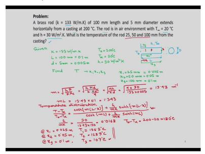
So, first problem is just first read. A brass rod with thermal conductivity 133 W/mK of 100 mm length and 5 mm diameter extends horizontally from a casting at 200 °C and the rod is in an air environment with  $T_{\infty}$  is 20 °C and heat transfer coefficient 30 W/m<sup>2</sup>K. What is the temperature of the rod 25, 50 and 100 mm from the casting okay?
