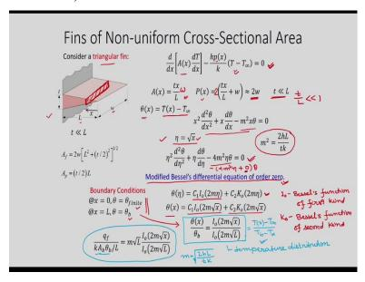
So, next now we will consider one fin with non-uniform cross-section okay. So, as these analysis is very cumbersome so will not go into details, just I will tell you the steps and how to find it and what is the final expression of the temperature distribution as well as the heat transfer rate. So, let us consider first one fin with non-uniform cross section and will consider a simplified fin that is our triangular fin.
